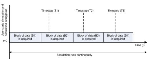
Asynchronous Analog Input – Scenario 2
