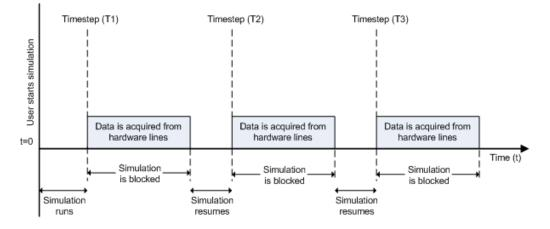
At the first time step (T1), data is acquired from the selected hardware lines. The simulation does not continue until data is read from all lines.
