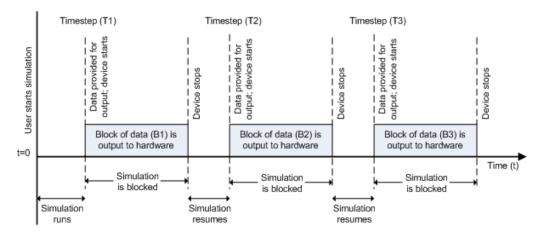
At the first time step (T1), data output is initiated and the corresponding block of data (B1) is output to the hardware. The simulation does not continue until B1 is output completely.
